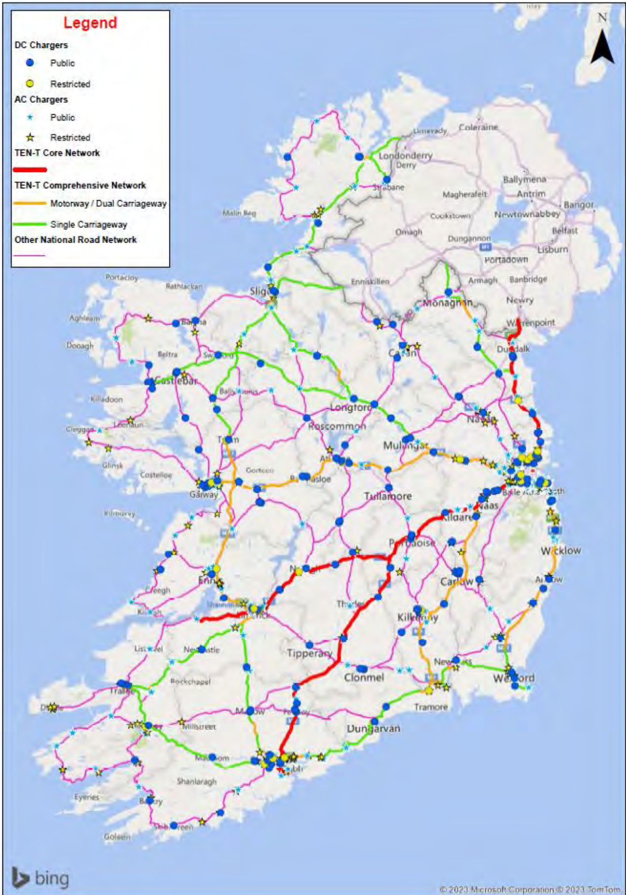
Figure 5.6 Current EV charging infrastructure on the National Road Network | NRNEVCP; Fig. 6
